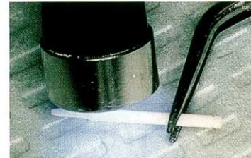
Figure 8—The adhesive was then light-cured for 10 seconds.
