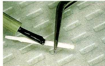
Figure 7—Adhesive (in two coats) was applied to the decontaminated post.
