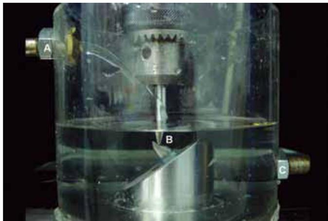
**5** Fracture resistance test performed in water circulation device. A, Water input. B, Wedge-shaped tip. C, Water output.
