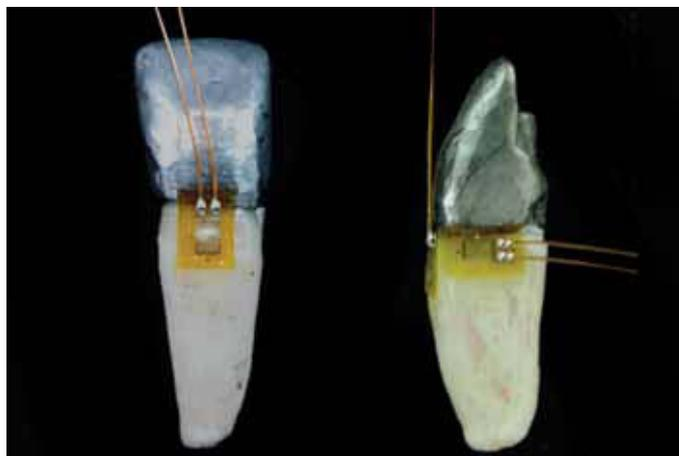
**4** Strain gauges attached at coronal cervical limit on buccal and proximal surfaces.
