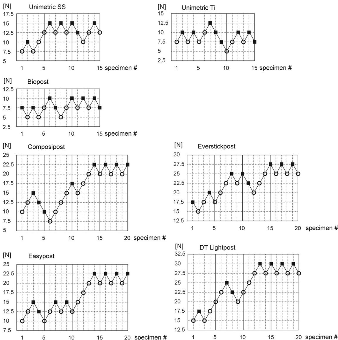
**Fig. 3 – Staircase data for the post-cement combinations investigated. The number of specimens in each series was increased in sets of five until five reversals were observed. This required 15 specimens for the ceramic and metal posts groups and 20 for the fibrous posts groups.**
