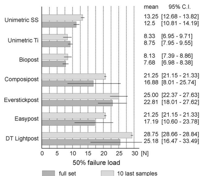
**Fig. 4 – Mean and 95% confidence intervals of the post-cement combinations tested. Results are given for the full data set (15, respectively 20 samples) and for a subset comprising only the last 10 samples of each series. Note the important decrease in standard deviation when only the last 10 samples are considered.**
