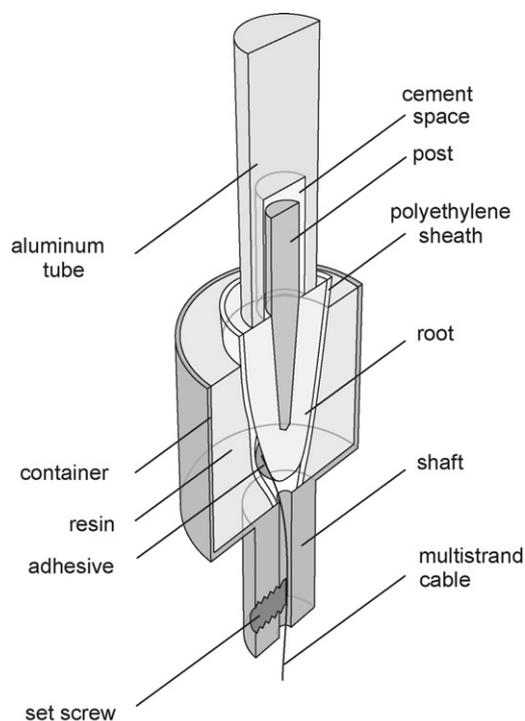
**Fig. 2 – Schematics of the specimens. The root was sheathed into a polyethylene hose and encased into resin (i.e. the bone analog). The resin was housed in a container featuring a shaft to be gripped into a rotating collet. The root was prevented from escaping its resin housing by a multistrand cable that was crew-fastened to the shaft. An aluminum tube that was cemented onto the post's head served as crown analog.**
