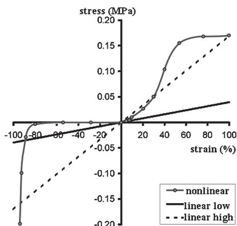
FIG. 4. Nonlinear stress strain curve for PDL. Stress is shown in MPa and strain in %.
