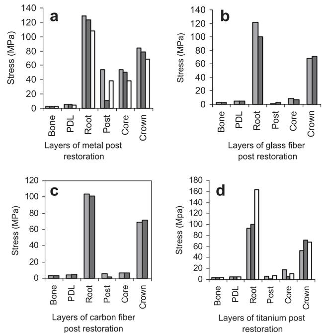
FIG. 6. Axial stresses on different layers of restoration. Graphs a–d show a comparison of stresses for the different domains of the tooth for different shapes of (a) the cast metal post, (b) glass fiber post, (c) carbon fiber post and (d) titanium post restoration. The threading in the fiber post is not feasible and hence stress values obtained using fiber posts are not considered for graphical comparison. Bars: light grey, parallel post; dark grey, tapered post; white, threaded post.
