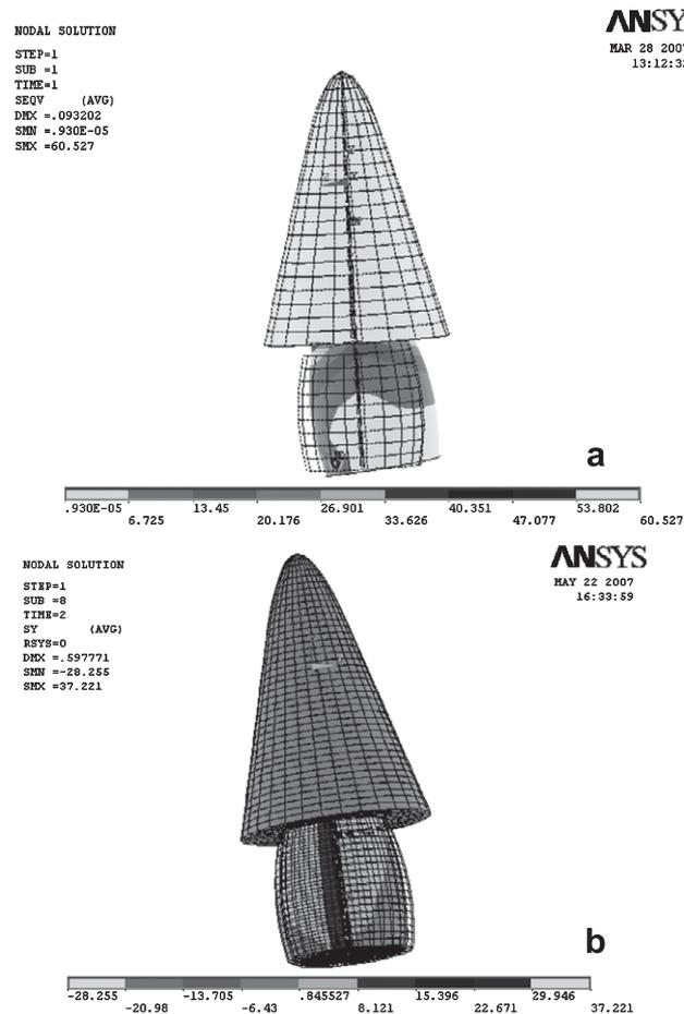
FIG. 7. Axial stresses on geometrically simplified assembly of restored maxillary central incisor: (a) linear analysis and (b) nonlinear analysis. Deformed and undeformed shapes of the crown are also shown.
