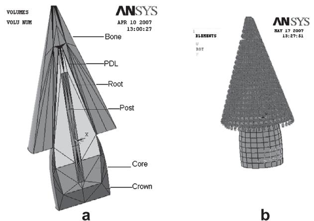
FIG. 3. Geometrically simplified model of restored tooth prepared in ANSYS. (a) Simplified model prepared for nonlinear analysis. The five layers are the bone, PDL, root, post and core, and crown. (b) Model loaded and constrained. A load of 200 N is distributed on the four nodes. The outer surface of the bone is constrained.
