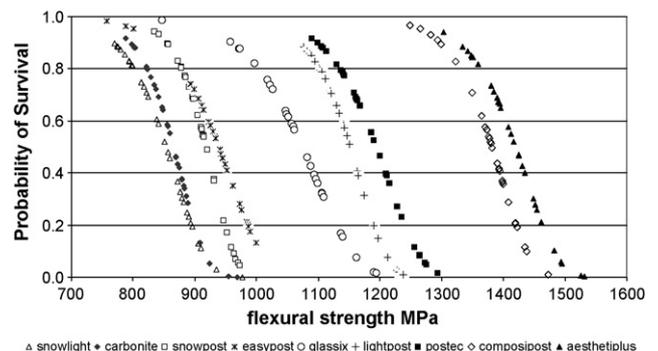
**Fig. 1 – Plot of flexural strength against survival probability for the FRC post materials.**
