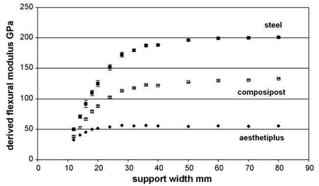
**Fig. 4 – Flexural modulus values calculated from three-point bend testing at decreasing support widths for steel, Composipost and Aesthetiplus samples.**
