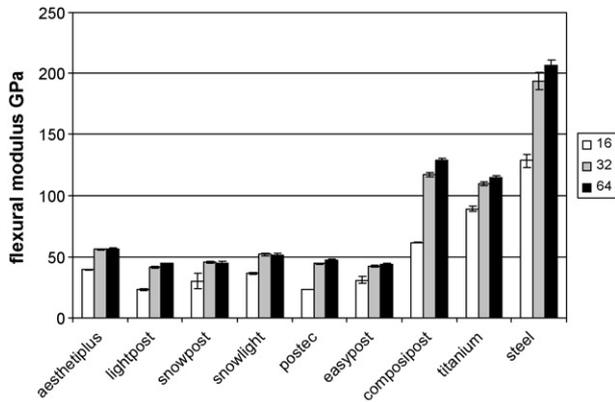
**Fig. 2 – Flexural modulus values (GPa) for the FRC and metal materials calculated from three-point bend testing at support widths of 16 mm, 32 mm and 64 mm. Errors bars indicate standard deviations.**
