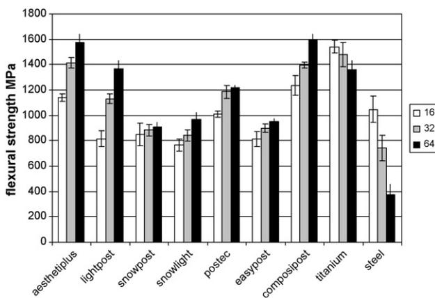
**Fig. 3 – Derived flexural strength values (MPa) for the FRC and metal materials at support widths of 16 mm, 32 mm and 64 mm. Errors bars indicate standard deviations.**
