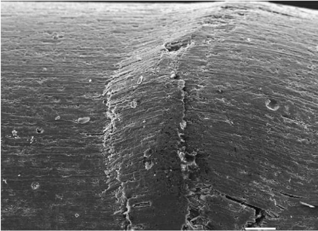
**Fig. 2** – S.E.M. photograph of carbon fibre post stored at 37 °C for 1 year, after fracture in three-point bend testing showing upper compression aspect of post with buckling and rupture of fibres.
