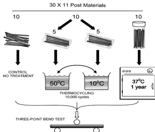
**Fig. 1 – Diagram of experimental set-up for treatment of posts and three-point bend testing.**
