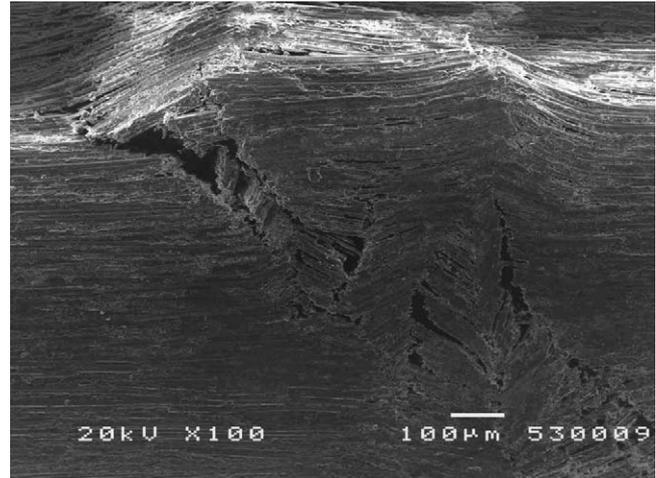
**Fig. 4** – S.E.M. photograph of fractured glass fibre post showing similar appearance of broken fibres on the upper compressed surface as seen with the carbon fibre post.
