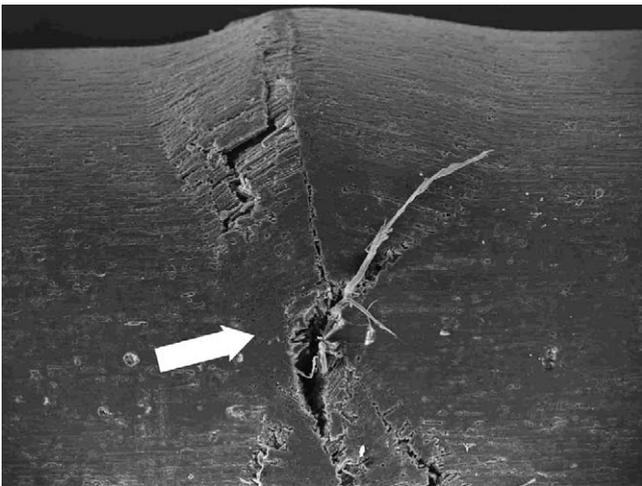
**Fig. 3** – S.E.M. image of fractured carbon fibre post showing point of application of three-point bend indenter (arrowed) with buckling and splitting of fibres on either side.
