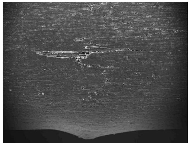
**Fig. 5** – S.E.M. photograph of lower (tension) surface of thermocycled glass fibre post sample after three-point bend testing, showing a small area of fractured fibres lifting out of the surface of the post with some cracking of the matrix evident which extends peripherally.
