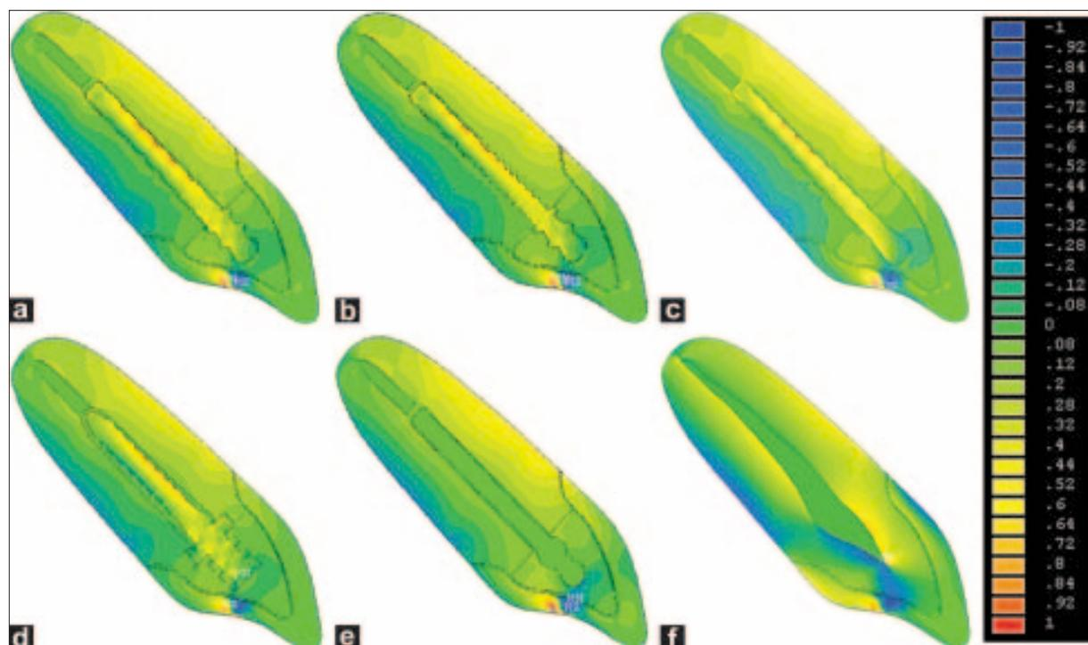
**Figure 3:** Stress distribution by shear stress criteria on maxillary central incisor models: (a) model XH; (b) model XT; (c) model XP; (d) model FF; (e) model FL; (f) model C
