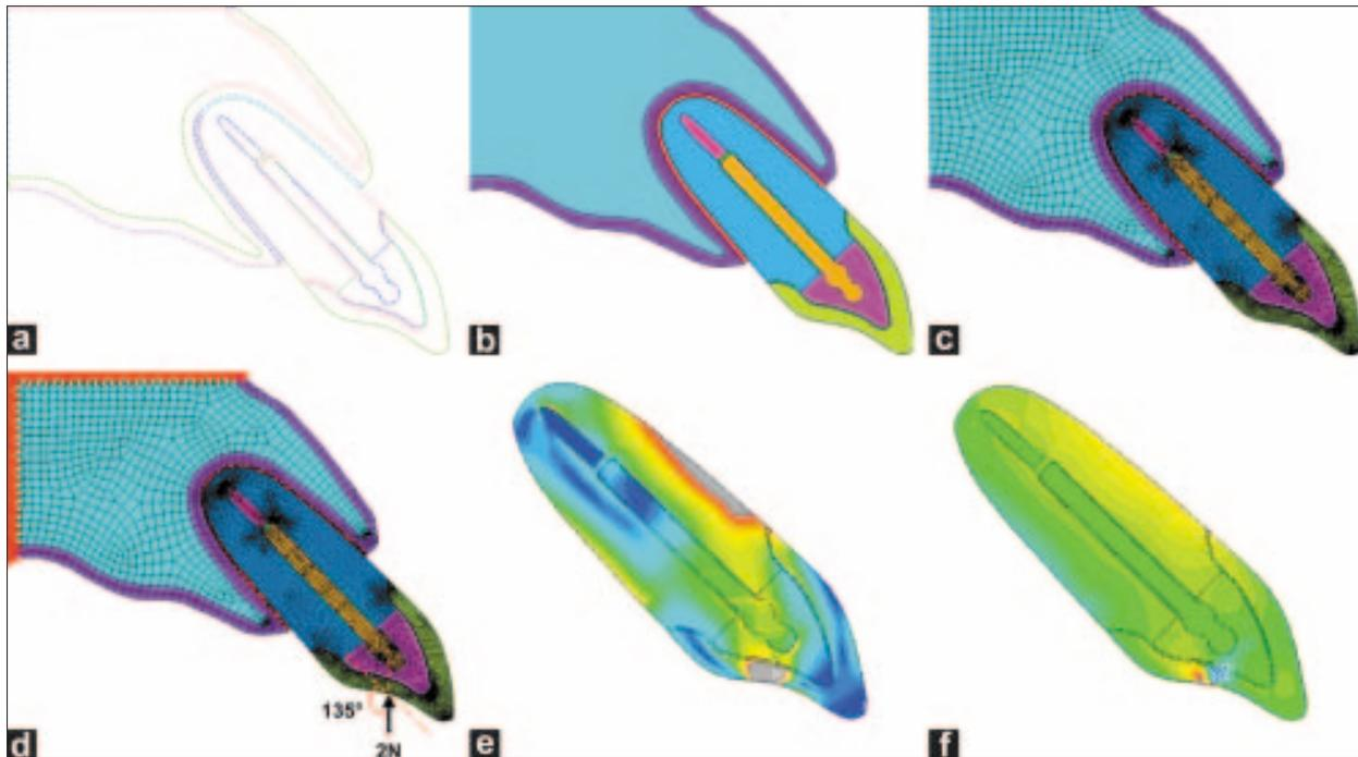
**Figure 1:** (a) Contours generated; (b) areas plotted for each structure and materials; (c) mesh of each structure; (d) model displacement restriction and load application; (e) stress distribution by von Mises criteria; (f) stress distribution by shear stress criteria
