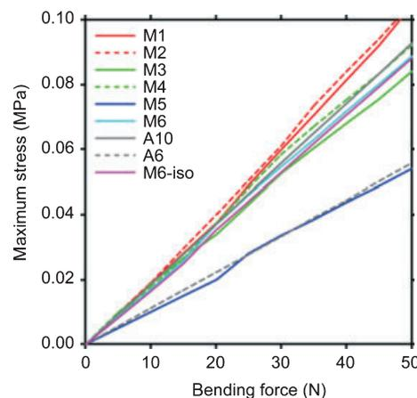
**Figure 3** Force–stress curves for the six bending models. The stress was the maximum flexural stress found at the bottom of the beams. Also shown are the analytical curves for a cylindrical beam calculated for 6 and 10 mm support span distances (diameter 1.9 mm).
