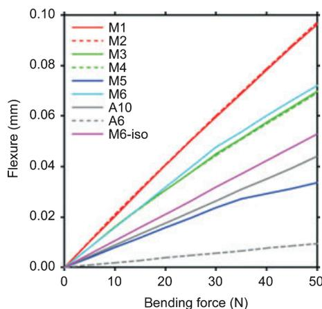
**Figure 2** Force–displacement curves for the six bending models. The flexure was determined at the load application point. Also shown are the analytical curves for a cylindrical beam calculated for 6 and 10 mm support span distances (diameter 1.9 mm).
