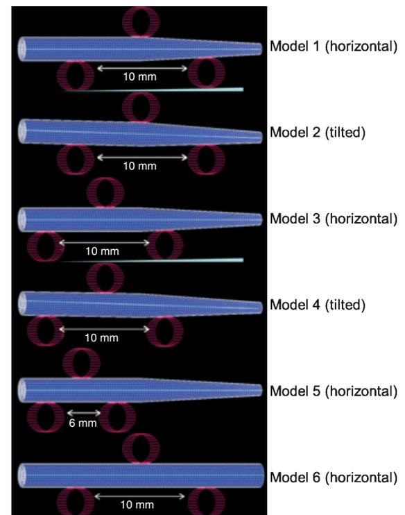
**Figure 1** Schematic illustration of 3D-models of the simulated three-point bending tests, showing the different placements, support distances and tilts.
