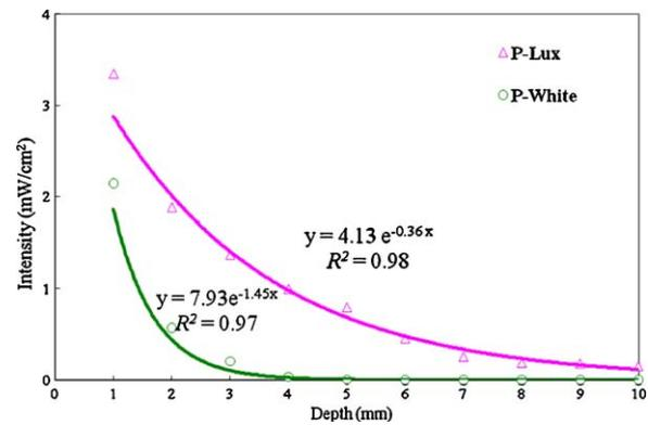
Fig. 3 – Light attenuation (at 470 nm wavelength) as a function of depth along two aesthetic posts.
