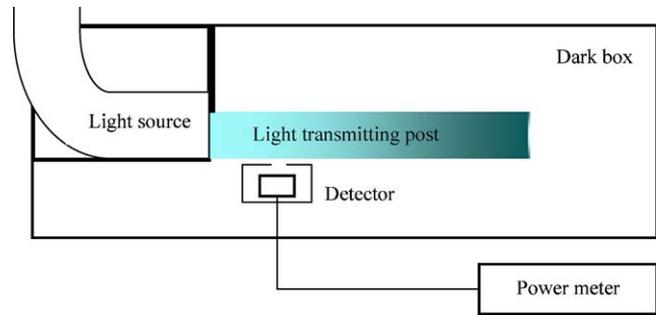
**Fig. 1 – Schematic illustration of radiance measurements along the post using a power metre. The light curing unit was attached to the top of the post in such a way that the post was the only path through which light could pass into the dark box.**
