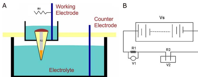
**Fig. 2 – Schematic drawing of (A) the electrochemical test apparatus and (B) the circuit diagram. Vs: 6.2 V; R1: 50.2 k $\Omega$ ; R2: impedance of the specimen.**
