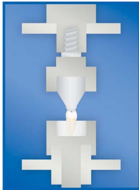
Figure 2. The schematic illustration of specimens in the load cycling machine.
