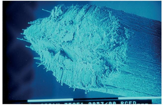
FIG 2. Cutting procedure with scissors. Two planes and convergent flanges are visible ( $\times 36$ ). Loss of integrity and morphology of the post is clearly noted.
