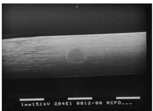
Fig. 5 A sample from Group 4, whereby the post remained unbroken after 2,000,000 cycles. Contact area with the loading punch is evident.
