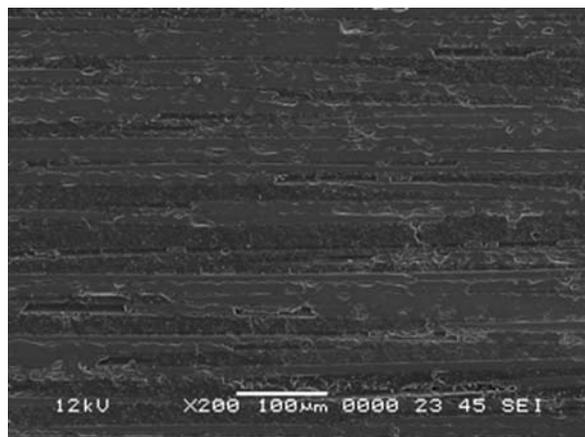
Fig. 3 Surface of Group 1 sample after the longitudinal cut.
