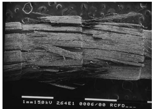
Fig. 4 A sample from Group 3, whereby post was fractured after fatigue test.
