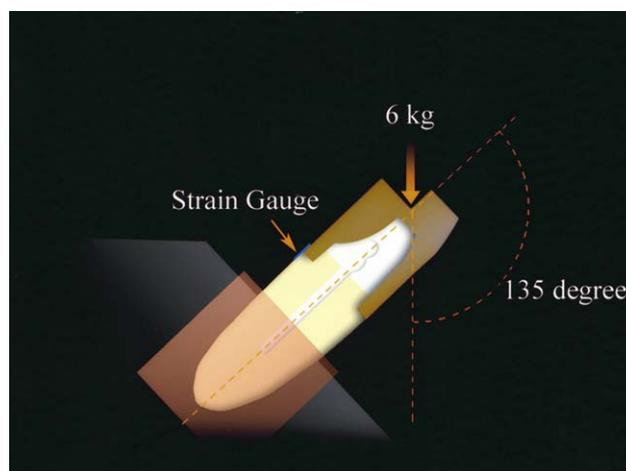
**Fig. 2.** Load value, load application angle, holding device, and strain gauge location.
