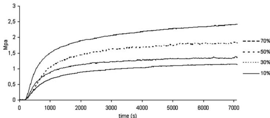
**Figure 1.** Representative curves of stress expressed in MPa of the different cements tested in the study during light exposures (sec).
