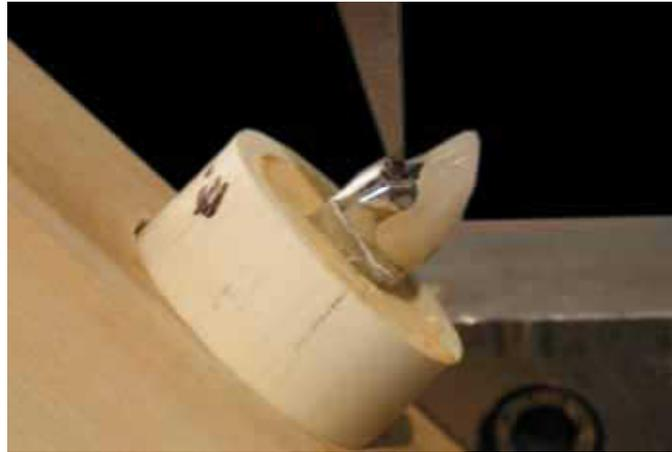
**2** Post-and-crown restored tooth secured in jig and testing machine to receive load.
