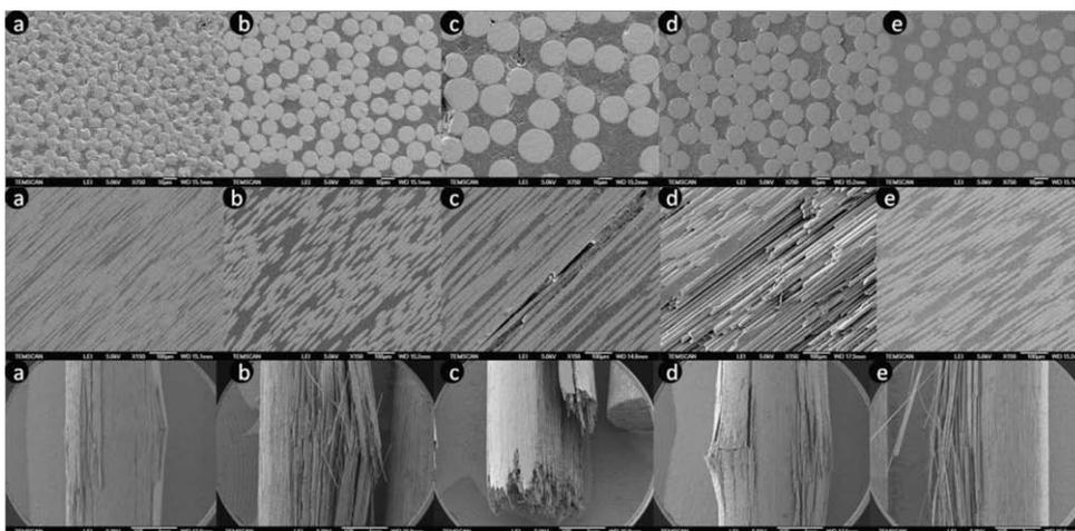
Fig. 1. SEM micrographs of the fiber posts (a, Aestheti-Plus; b, Light-Post; c, Snowpost; d, Snowlight and e, FRC Postec). Upper line: transverse section, magnification 750, bar = 10  $\mu\text{m}$ ; middle line: longitudinal section, magnification 150, bar = 100  $\mu\text{m}$ ; lower line: failure mode, magnification 25, bar = 1 mm.
