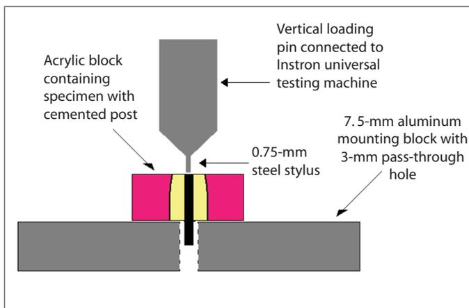
**Fig 1** Schematic drawing of a mounted specimen with cemented post and vertical loading apparatus.
