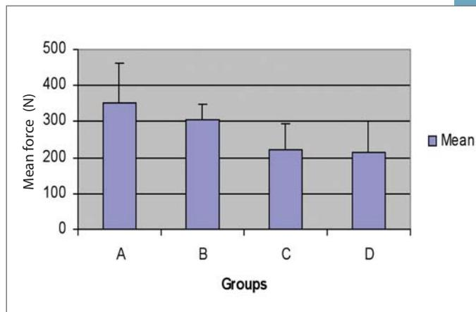
**Fig 2** Mean force (N) required to dislodge posts in each group. The height of each bar represents the mean and the brackets represent  $\pm$  SE.
