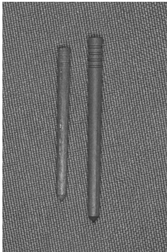
Figure 1 Carbon fiber-reinforced epoxy resin dowels.
