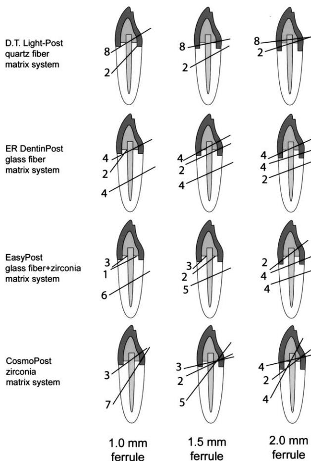
**Fig. 4.** Locations and frequencies of fractures in 4 test groups.
