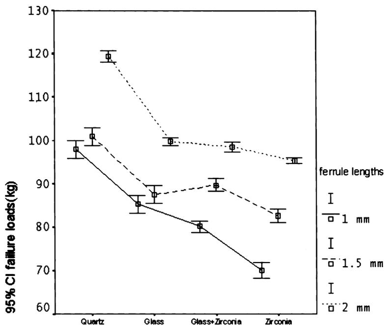
**Fig. 3.** Failure thresholds for specimens prepared at ferrule lengths of 1.0 mm, 1.5 mm, and 2.0 mm, and restored with 4 different dowel systems.
