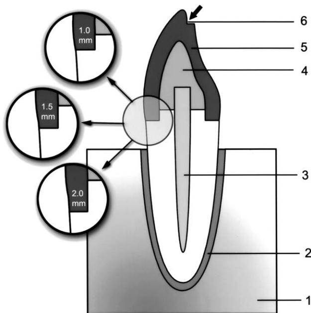
**Fig. 2.** Schematic drawing of specimen mounted in acrylic resin block and illustration of ferrule effect: 1, resin block, 2, silicone simulated periodontal ligament, 3, prefabricated dowel, 4, composite core, 5, cemented metal crown, and 6, arrow indicating 130-degree angle load applied to prepared step on palatal surface.
